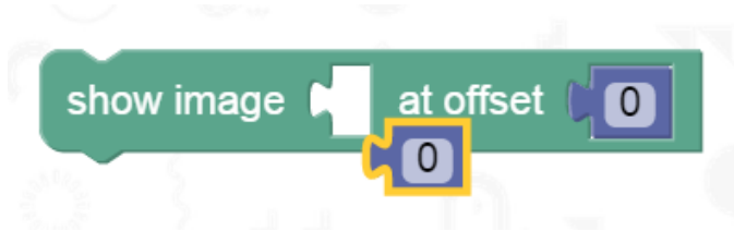
Fig. 2. Blockly's UI prevents connecting these two blocks: the "show image" block is defined as taking an image, not a number.
