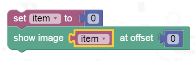
Fig. 3. This program cannot be translated to valid C++, since the item variable cannot be both an integer and an image.
